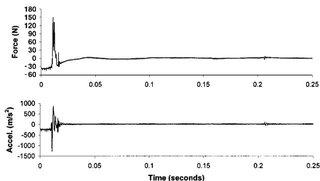
**Fig 3.** Load and acceleration characteristics of a typical SMT delivered by the AAI II. Note that the force-time history produced by the AAI II is associated with a short duration (<1 ms), high loading rate, and impulsive force signal.
